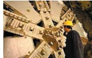
Shield of the tunnel boring machine.
