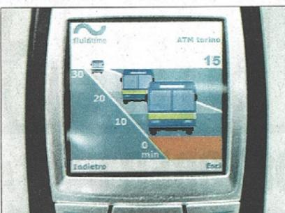
This Internet-connected wristwatch (which was jury-rigged by the fluidtime team) features little buses passing time markers in the road to show and tell testers when their bus (and the one after it and the one after that) is set to arrive at their chosen stop.
